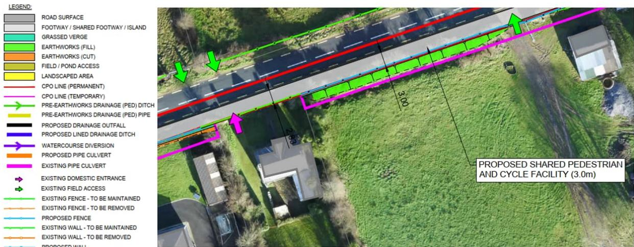
Figure 4-5 Close up of boundary details from EIAR Figure A4.13 with Legend included
